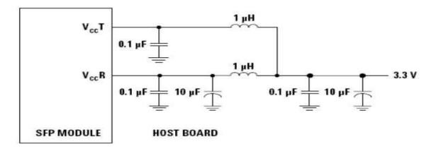
Note: Inductors with DC resistance of less than1Ωshould be used in order to maintain the required voltage
