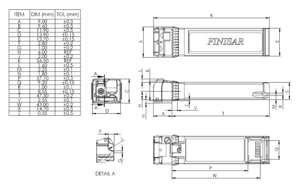
Figure 2. FTLX2672D327/FTLX2672D333 Mechanical Dimensions
